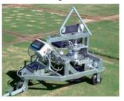
The spiked disc and the options listed above should be considered to provide common indicators of horizontal surface shear resistance.
